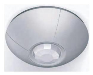
The LOS-CIR Series ceiling-mount passive infrared sensors can integrate into Lutron systems or function as standalone controls using a Lutron power pack. The sensor uses a small semiconductor heat detector that resides behind a multi-zone optical lens. The sensor's detector is sensitive to the heat emitted by the human body. In order to trigger the sensor, the source of heat must move from one range of detection to another. Non-moving hot objects will not cause the lights to turn on.
