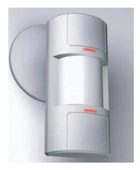
The LOS-WIR wall-mounted passive infrared sensor is used in spaces with pendant fixtures, ceiling fans, or high ceilings (more than 12 ft./3.7 m). The sensor detects large body motions over 40 ft. (12 m) away, and smaller motions such as hand movements up to 25 ft. (7.6 m) away.
