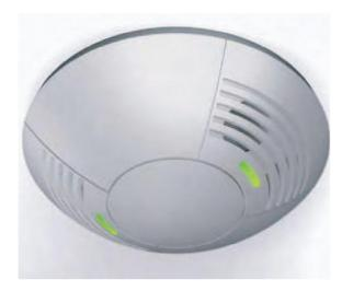
The LOS-CUS Series ceiling-mount ultrasonic sensors can integrate into Lutron systems or function as stand-alone controls using a Lutron power pack. Any movement within the sensor's range causes a shift in the original emitted frequency. The sensor's receiver identifies any change in frequency as motion and either turns the lights on or maintains lights on.
