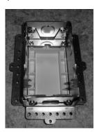
Push the front box section down until the leveling fixture makes full contact with the flat surface. Next, push the mounting ring down until it makes full contact with the back of the stone. Holding both parts down firmly, tighten the four screws between the front box section and the mounting ring.
