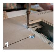
Remove the mud dam from the mounting platform
