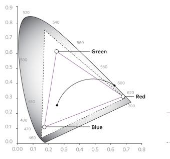
Ketra's D4R LED Downlight can easily be commissioned into Lutron HomeWorks or Athena systems. The product can reproduce any color point within the triangle shaped gamut indicated in the chart to the left. With Ketra's innovative optical and thermal feedback system, the color point is maintained to an accuracy of one-step MacAdam Ellipse over the lifetime of the product and across operating temperature range.
