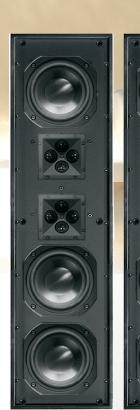
Size Custom h x 8.125 w x 3.875 d (in) 854 h x 206 x w 98 d (mm) depth w/arille 4.125 d(in) 104(mm) Freq Response 65Hz-24kHz±3dB Impedance 4/8 ohms (Config. Dependent) Sensitivity 89dB 2.83V / 1m Power reg. 50-200W/Channel Woofer (3) 5.25" (133mm) Aluminum Tweeter (8) 0.75"(19mm) Aluminum Finishes White Paintable Grille (Paintable by Request Only) PCB OX5CSPB PCBF OX5CSPBF
