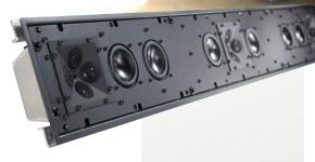
Size 7.269 h x Custom w x 3.875 d (in) 184.5 h x 991 w x 98 d (mm) Freq Response 70Hz-24kHz±3dB Impedance 4/8 ohms (Config. Dependent) Sensitivity 89dB 2.83V /1m Power req. 25-150W/Channel Woofer (4) 3" (76mm) High Excursion Tweeter (8) 0.75"(19mm) Aluminum Finishes White Paintable Grille (Paintable by Request Only) PCB QX3LRPB PCBF OX3LRPBF
