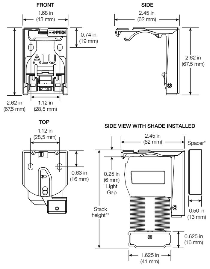
\* Spacers are included when outside-mount above/below trim is indicated on the original order, and/or the shade is equipped with an external battery holder.
