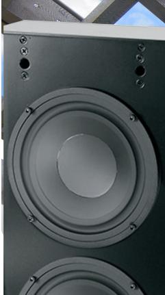
Size 40 h x 8.125 w x 4" d (in) 1016 h x 206 w x 102 d (mm) Freq Response 60Hz-40kHz±3dB Impedance 4 ohms Sensitivity 96dB 2.83V /1m Power req. 25 -200 watts Woofer (4) 6.5" (165mm) Aluminum Tweeter (4) 1" (25mm) Titanium Quad-array Mount Through Hole (Optional Brackets) Finishes Gloss White, Satin Black, or Custom
