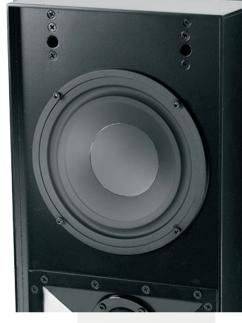
Size27 h x 8.125 w x 4" d (in)<br/>685 h x 206 w x 102 d (mm)Freq Response65Hz-40kHz±3dBImpedance4 ohmsSensitivity95dB 2.83V /1mPower req.25 -200 wattsWoofer(2) 6.5" (165mm) AluminumTweeter(4) 1" (25mm) Titanium Quad-arrayMountThrough Hole (Optional Brackets)FinishesGloss White, Satin Black,<br/>or Custom
