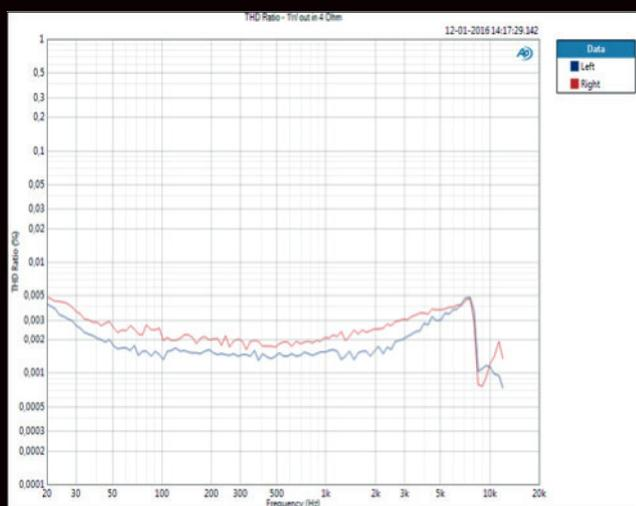
The Total Harmonic Distortion (THD) of the amplifier is below 0.005% across the audio bandwidth 20-20 kHz measured at 1W output power into 4Ω. At 30W output power the amplifier meets THD levels between 0.015% and 0.03% successfully independent of frequency.
