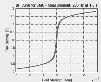
Graphs are showing the hysteresis on iron based magnets in relation to SMC. There is almost no hysteresis, and therefore no distortion using SMC.
