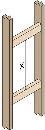
3. Place space saver, preconstruction zip ring bracket, or both in desired speaker location. See page 4 for when to use space savers and zip rings. Space savers are recommended for every new construction project. Zip rings are recommended as a time-saver on very large projects with dozens of invisible speakers.
