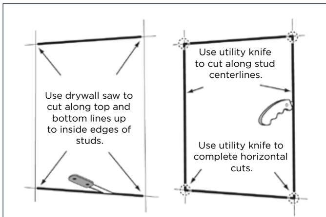
6. Remove drywall from opening. This should expose only 3/4" (19mm) of each stud/joist or half of the stud/joist surface. Remove any exposed drywall nails or screws.
