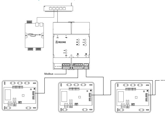
**Important:** The Webserver HUB can control up to 32 systems simultaneously from a single Lutron HomeWorks QS system. Each system has an identifier that will be necessary to perform the configuration through Lutron Designer.
