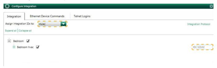
6. Click on the "Telnet Logins" tab on the Configure Integration screen. Enter the Username and Passphrase that will be used by the Webserver HUB to make the Telnet connection to the HomeWorks QS Processor.
