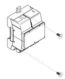
Note: To remove the module on DIN rail, pull the tab downwards to release it.
