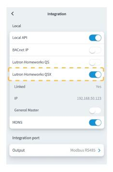
$After \ enabling \ integration \ with \ the \ Lutron \ HomeWorks \ QSX \ Processor, 3 \ parameters \ appear:$
