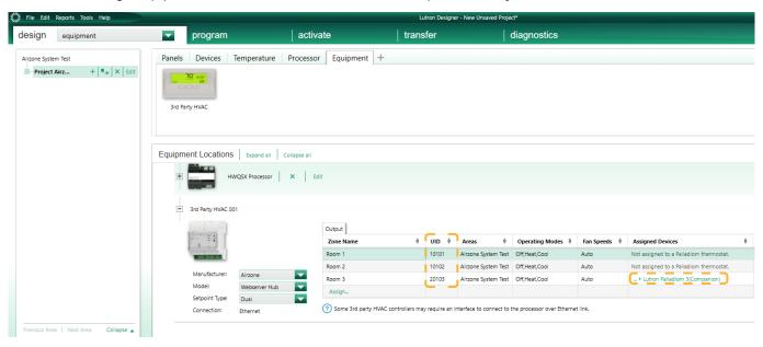
**Note:** The UID must be unique for each zone and will be assigned with the format 2XXYYY or 1XXYYY, depending on whether the zone has a Lutron Palladiom thermostat or not, as described on page 13.
