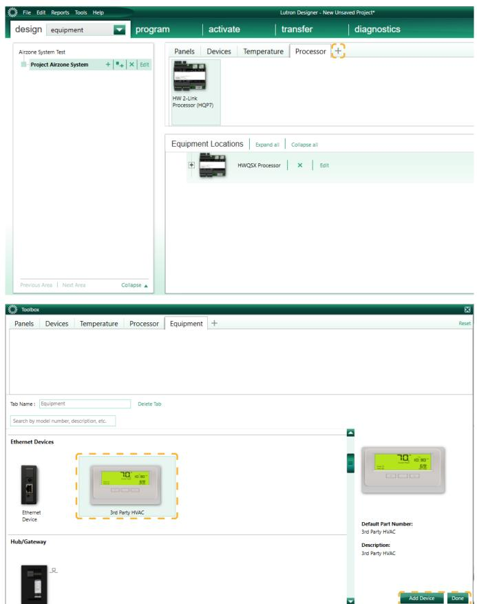
Once the device has been added, select "Airzone" in the *Manufacturer* drop-down menu, under *Model* select "Webserver HUB" and under *Setpoint type* select "Dual" for VAF/ZBS/ZS6 systems or "Single" for Flexa/Acuazone/RadianT systems.
