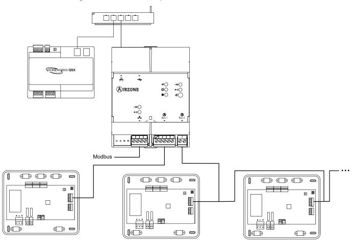
**Important:** The Webserver HUB can control up to 32 systems simultaneously from a single Lutron HomeWorks QSX system. Each system has an identifier that will be necessary to perform the configuration through Lutron Designer.
