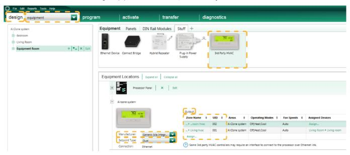
Once the device has been added, select "Generic (via integration)" in the *Manufacturer* drop-down menu and under *Setpoint type* select "Dual" for VAF/ZBS/ZS6 systems or "Single" for Flexa/Acuazone/RadianT systems.
