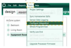
5. Select the *Integration* tab and, in the *Assign integration IDs* drop-down menu, click on "Devices". The *Integration IDs* of the Palladiom thermostats must now be assigned manually with the 2XXYY format as described on page 9.
