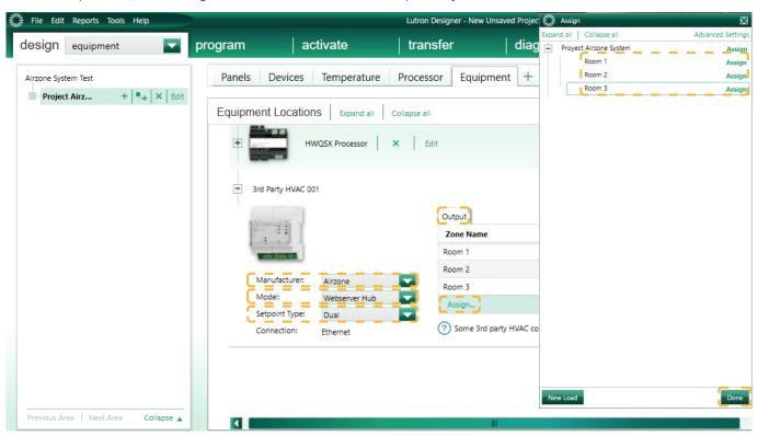
Set the minimum and maximum set point temperature to 19°C and 30°C (66°F and 86°F), respectively. In the case of "Set point Dual", set the "Minimum Heat/Cool Set point Difference" value equal to that of the Lutron system.
