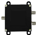
-7 dB Tap 700-2700 MHz w/1.5 dB Pass Thru 75 Ohm (F Connector) 859115*
