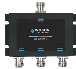
Splitter 3 Way -4.8 dB 700-2700MHz w/N Female Connectors, 50 Ohm 859980*
