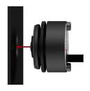
3) Twist the locking nut up against the depth nut to secure the sensor.
